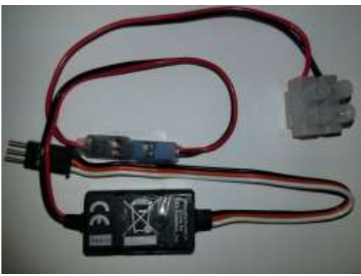
Motor Controller and Motor Cable (4)
